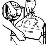
**4.** Push Side-Lock Latch down and tilt drawer side open.
