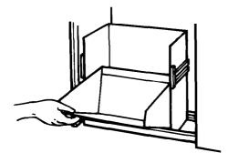
Hold Side-Lock Latch and tilt side of drawer until the latch clears the drawer front.
