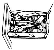
Bottles or cans not placed in the center may become caught between the ram and the drawer. The Drawer Monitor Switch senses a "misload" and causes the ram to return to the "up" position without compacting. Load bulky trash, bottles and cans in the **center** of the drawer.
